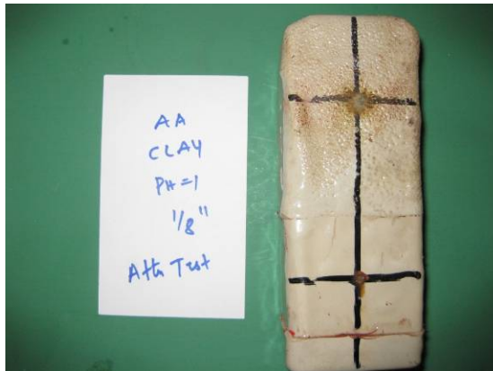
Figure 4-2. Clay brick holiday specimen exposed to 1% H 2 SO 4 solution.
